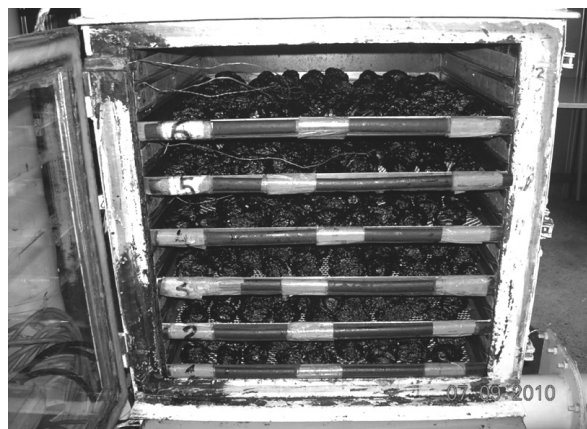
Sl. 1. Komora sušare sa lesama na kraju sušenja Fig. 1. Drying station chamber with trays at the end of the drying cycle
